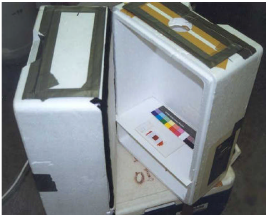
Figure 2. Detail of the light-box when opened to replace samples. Note the hole in the viewing port for mounting the camera.
