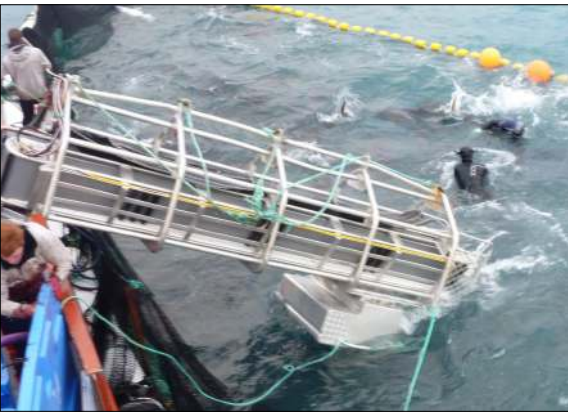
Hydraulic lifting conveyor
